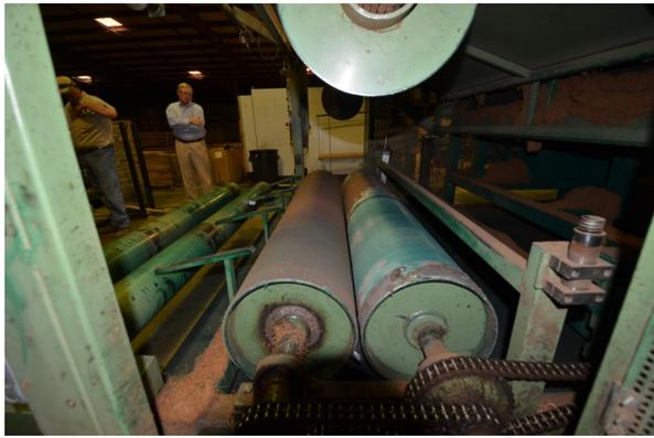
Drawing (at right) of a nip point in the ANSI Safety Standard for Mechanical Power Transmission Apparatus, ASME B15.1-1996. Photograph at left is of the winder rollers of Jimmy's machine.
